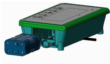
Install the battery housing.
